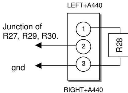
Switch SW2 viewed from behind (pins facing toward you). With switch in the up position (LEFT+A440) pins 2 and 3 are connected.
