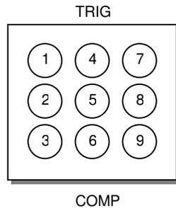
Switch viewed from behind (pins facing toward you). With switch in the up position (Trigger Mode) pins 2 and 3 are connected, pins 5 and 6 are connected, and pins 8 and 9 are connected.
