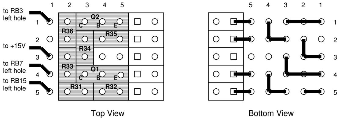
Use the following table to place components from the TLN-865 schematic onto board #3. For short jumpers, use a scrap resistor lead. For longer jumpers, use a piece of #22 wire. Watch the orientation of the diodes; the circuit won't work if you put them in backwards. Check the website pictures.
