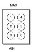
Switch viewed from behind (pins facing toward you). With switch in the up position (MAX) pins 2 and 3 are connected, and pins 5 and 6 are also connected.
