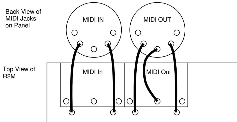
To hook up the manual to the TLN-854, you will likely need to create a new cable that has four conductors plus a shield. I call this the “manual cable”. USB cables are usually short and quite stiff. I found some great cable at a pro audio store. I don’t have a part number for it; it just says “MIDI CABLE” on the outside. It has a black outer casing and is quite flexible, just like instrument cable, but inside there are four conductors plus a shield.
